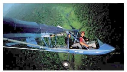
Air-Cam. Only 2 of this design were built by Leza Lockwood - 1 for National Geographic and this one that I own. The stats include: 1994, 2-seater, dual controls, open cockpit, twin Rotax 582's, 735TT, 45 SMOH, Royal blue fiberglass body, additional gas tanks; excellent condition. A blast to fly & land almost on a dime!! I have often circled "up close & personal" above the alligators in Lake Apopka. Price is \$43,500. Located in Orlando. Pete (407) 924-7109; email: joanne@atlantic.net.
